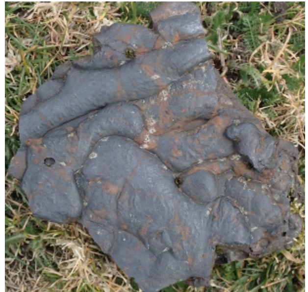
Figure 2: Example of tap slag from a mediaeval bloomery site near Clitheroe
