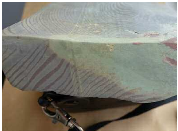
Moughton whetstone showing probably cleavage (horizontal plane) and bedding (vertical plane in the location where the Liesegang rings are disrupted)
