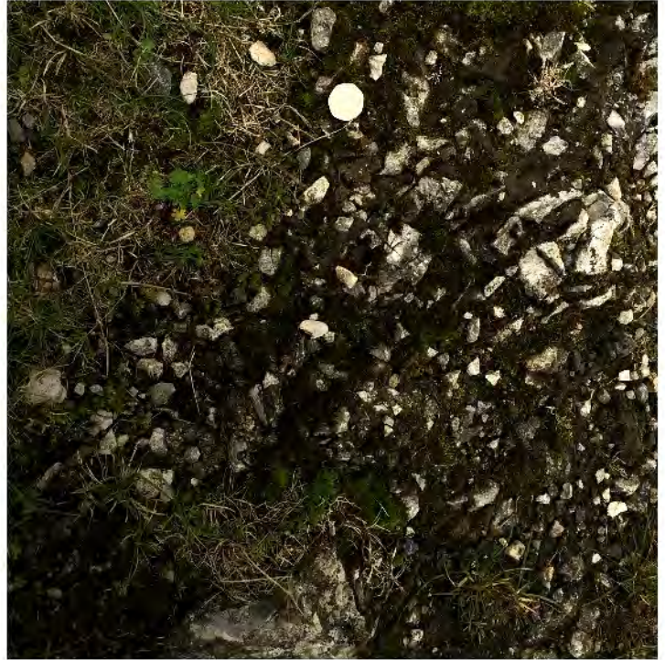
Fig. 7 Black bitumen can be seen filling the spaces, in stark contrast to the white limestone
