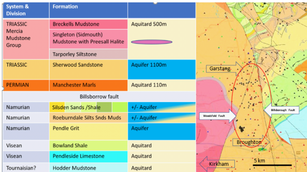
Figure 7 Stratigraphy and aquifer potential. Public water supplies are abstracted from within the red oval.
