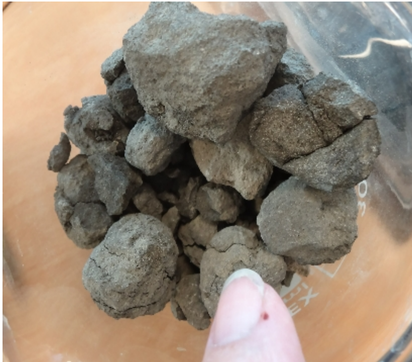
Fig 6. The clinker which is crushed to a fine powder to form the cement.
