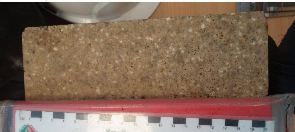
Fig 5. An example of a 220 mm fire brick that line the rotating kilns.
