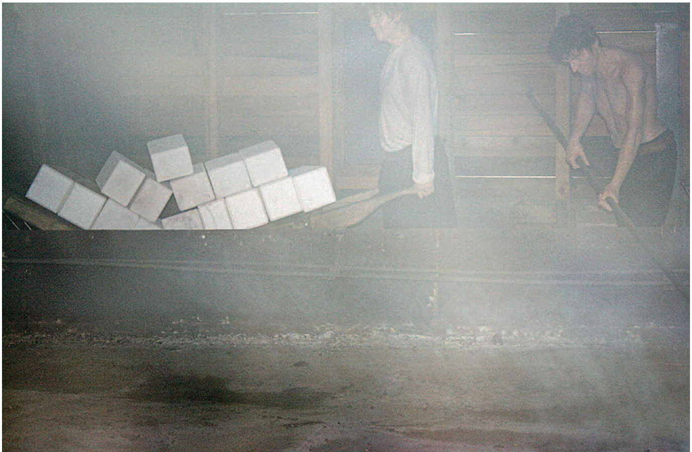
Fig. 3 Collecting salt from the open pan
