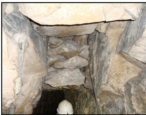
Stemples across the stope formed a platform for waste rock
