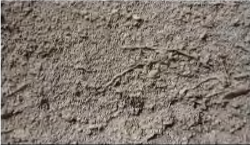
Figure 6: Portland Stone in the Manchester Cenotaph, St Peter's Square, showing ooliths and weathered-out fossils of bivalves
