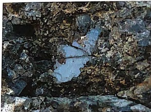
Figure 3 Localised zone of pegmatite containing coarse pyroxene crystals up to 5cm across
