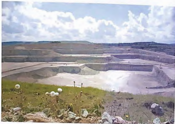
Figure 5. Viewpoint D. Old Moor Quarry. Note the drilling rig, with the line of holes awaiting explosives, taken in June 2009. Excavation of a further level will expose the Woo Dale Limestone.
