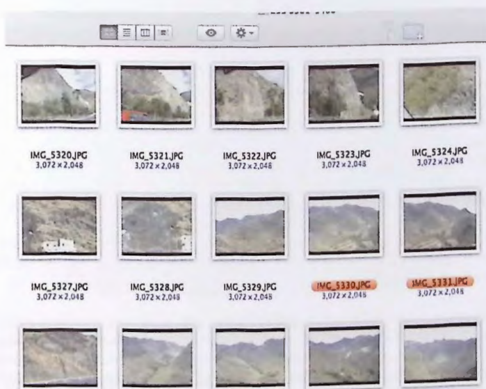
Figure 11. An array of image thumbnails, with a stereo pair at 5330 (RHS image) and 5331 (LHS image). Look at the pair cross-eyed to see the 3D effect.
