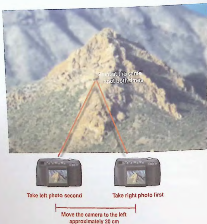
Figure 5. Take a stereo pair by taking two photographs consecutively, first to the right, and then to the left.
