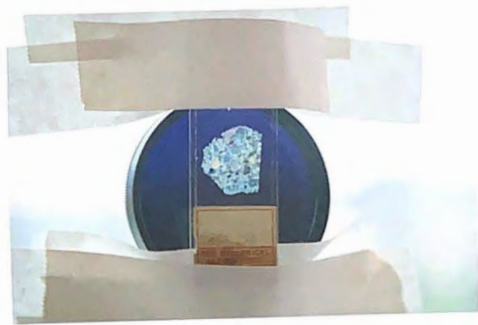
Figure 4. Mineral slide mounted in front of a circular polarising filter for a 35 mm digital camera.
