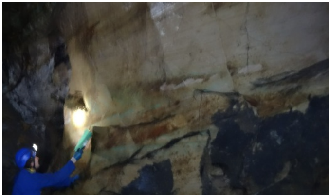
The primary copper deposits are concentrated in the foresets. This is because the grains making up the foresets are graded from fine to coarse. The coarse sections are more porous than the fine sections allowing the mineralising fluids to flow through and depositing the copper as they pass. Above are sections within the mine and below left is a sample.
